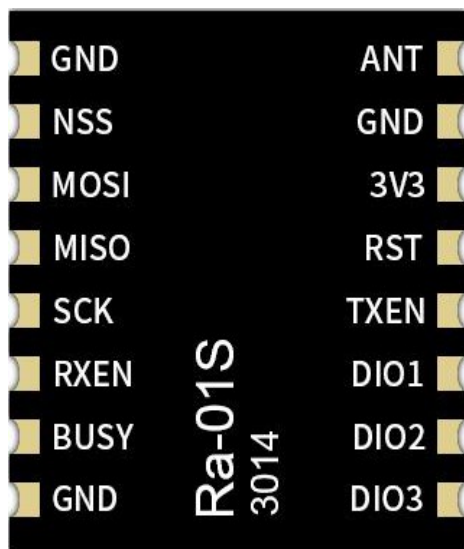
Ra-01SC Pin diagram
