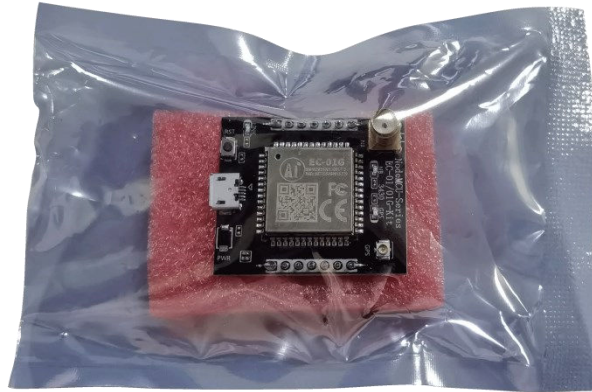
Figure 11 Packing diagram of an ESD bag
